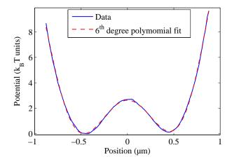
Figure 4: Double well potential measured by computing the equilibrium distribution of one particle's positions, with  $I_{\text{laser}} = 15 \text{ mW}$ . Here the distribution is computed on 1.5e6 points sampled at 502 Hz(i.e.a50 minlong measurement). The double well potential is well fitted by a 6<sup>th</sup> degree polynomium.
