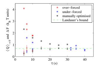
Figure 10: Mean dissipated heat (\*) and effective free energy difference (×) for several procedures, with fixed  $\tau$  and different values of  $f_{\text{max}}$ . The red points have a force too high, and a  $P_{S \text{ force}} \geq 99\%$ . The blue points have a force too low and  $91\% \leq P_{S \text{ force}} < 95\%$  (except the last point which has  $P_{S \text{ force}} \approx 80\%$ ). The black points are considered to be optimised and have  $95\% \leq P_{S \text{ force}} < 99\%$ .
