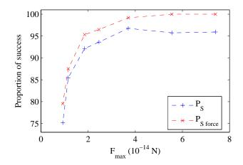
Figure 7: Proportion of success for different values of  $\tau$  and  $f_{\text{max}}$ , keeping constant the product  $\tau \times f_{\text{max}} \approx 0.4 \text{ pN s}$  (which corresponds to  $\tau \times v_{max} =$  $20 \,\mu\text{m}$ ).  $P_S$  quantifies the ratio of procedures which ends in state 0 after the barrier is risen.  $P_{S \text{ force}}$  quantifies the ratio of procedures which ends in state 0 before the barrier is risen.
