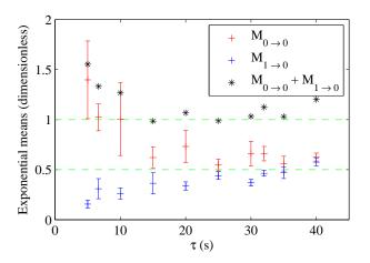
Figure 11: Exponential means computed on the sub-procedures, for several parameters, with fixed  $\tau$  and manually optimised values of  $f_{\text{max}}$ . The errorbars are estimated by computing the exponential mean on the data set with 10% of the points randomly excluded, and taking the maximal difference in the values observed by repeating this operation 1000 times.
