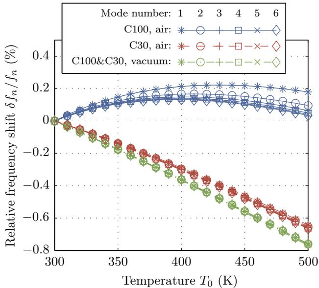
FIG. 9. (Color online) — Theoretical relative frequency shift  $\delta f_n/f_n$  versus uniform temperature  $T$  of cantilever and air according to the Sader model. The shift is the sum of two opposite effects when temperature rises: the softening of the cantilever (only effect in vacuum), and the decreasing of the inertial effects due to the surrounding atmosphere. The latter effect is dominant for the wider cantilever at low  $T$ . For a uniform temperature, the mode dependency is weak.
