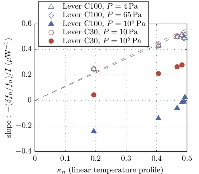
FIG. 4. (Color online) — Slope of the relative frequency shift versus light power as a function of coefficient  $\kappa_n$  (expected mode dependence for a linear temperature profile). The proportionality (dashed lines) is reasonable for both cantilevers in vacuum. At atmospheric pressure, a global vertical offset (mode independent contribution) can be observed.
