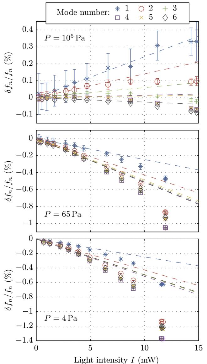
FIG. 2. (Color online) — Cantilever C100: relative frequency shift  $\delta f_n/f_n$  for modes  $n = 1$  to  $6$  as a function of the incident light power  $I$  on the lever, at atmospheric pressure  $P = 10^5$  Pa, top) and in vacuum ( $P = 65$  Pa middle,  $P = 4$  Pa bottom). The dashed lines are linear fits on the initial part of the curves ( $I < 6$  mW). The curves shapes are nonlinear, and depends strongly on pressure and mode number.
