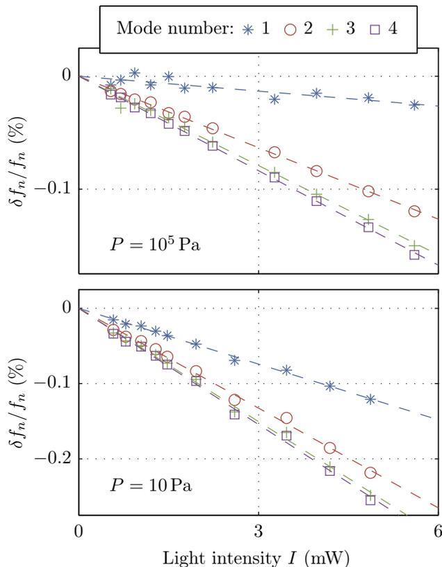
FIG. 3. (Color online) — Cantilever C30: relative frequency shift  $\delta f_n/f_n$  versus incident light power  $I$  on the lever, at atmospheric pressure  $P = 1 \times 10^5$  Pa, top) and in vacuum ( $P = 10$  Pa bottom). The dashed lines are linear fits.
