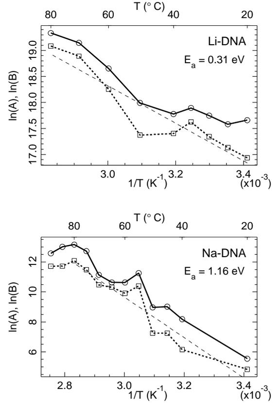
**Fig. 11.** Arrhenius plots of the coefficients  $A$  and  $B$  modeling the conductivity, i.e. plot of  $\ln A$  (open circles),  $\ln B$  (open squares) versus  $1/T$ , where  $T$  is the absolute temperature in Kelvin. Top panel: Li-DNA film, bottom panel: Na-DNA film. The oblique dash line corresponds to the linear fit of the temperature dependence of these quantities.
