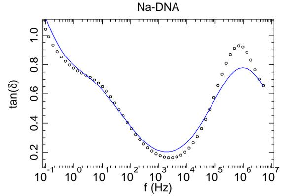
**Fig. 9.** Loss tangent  $\tan \delta = \epsilon''/\epsilon'$  versus frequency for the Na-DNA film at  $T = 20^\circ\text{C}$ . The points are the measurements and the line shows the theoretical fit with Eq. (1).
