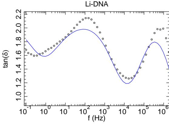
**Fig. 5.** Loss tangent  $\tan \delta = \epsilon''/\epsilon'$  versus frequency for the Li-DNA film at  $T = 20^\circ\text{C}$ . The points are the measurements and the line shows the theoretical fit with Eq. (1).
