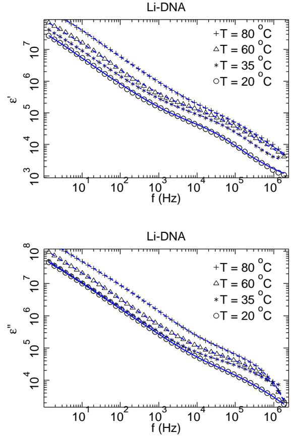
**Fig. 2.** Variation of the real (top panel) and imaginary (bottom panel) parts of the dielectric response function  $\epsilon^*(f)$  of the Li-DNA film versus frequency at different temperatures. The points are the measurements and the lines show the theoretical fits discussed in 3.2.
