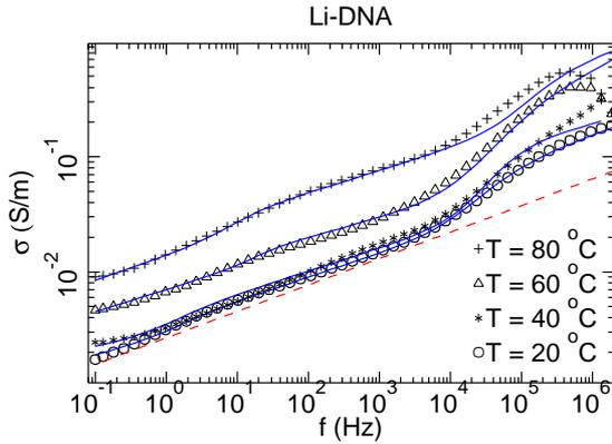
**Fig. 4.** Variation of the conductivity  $\sigma(f)$  of the Li-DNA film versus frequency at different temperatures. The points are the measurements and the full (blue) lines show the theoretical fits discussed in Sec. 3.2. The (red) dash line is a guide to the eye to illustrate the deviation from a simple power law at  $T = 20^\circ\text{C}$ .
