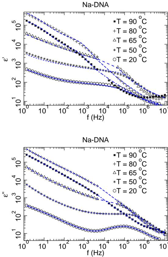
**Fig. 7.** Variation of the real (top panel) and imaginary (bottom panel) parts of the dielectric response function  $\epsilon^*(f)$  of the Na-DNA film versus frequency at different temperatures. The points are the measurements and the lines show the theoretical fits discussed in 3.2.
