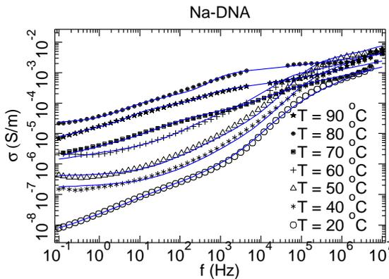
**Fig. 8.** Variation of the conductivity  $\sigma(f)$  of the Na-DNA film versus frequency at different temperatures. The points are the measurements and the full (blue) lines show the theoretical fits discussed in Sec. 3.2.
