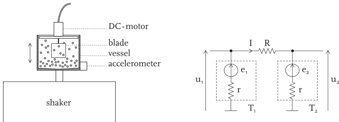
**Figure 1.** On the left, one of the two ensembles shaker + vessel + motor + blade. The motor + blade ensemble is fixed on a cover. On the right is the electrical circuit of the compound system. The motors are schematized by voltage sources ( $e_i \propto \dot{\theta}_i$ ) and the internal resistances  $r$ .
