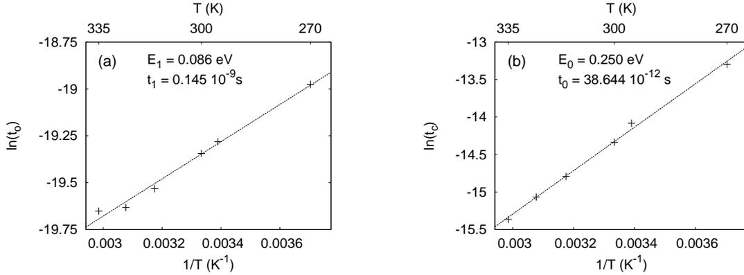
**Fig. 8.** Arrhenius plot of the duration of the open state  $t_o$  (a) and of the lifetime of a closed base pair  $t_c$  (b) in the model with a barrier in the intra-pair potential. The figure shows  $\ln(t_o)$  and  $\ln(t_c)$  versus  $1/T$ .
