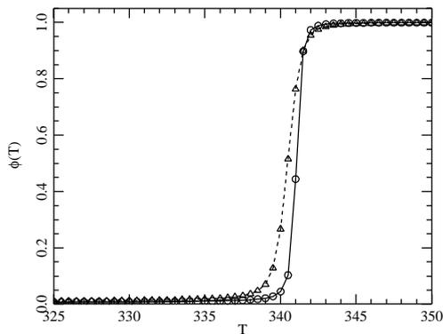
**Fig. 5.** Comparison of the melting profiles for poly-A DNA sequences computed with the modified PBD model with a closing barrier (full line with circles) and the PBD model with the Morse potential (dotted line with triangles)
