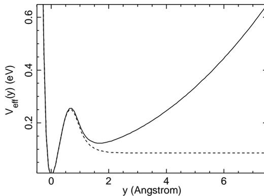
**Fig. 13.** Effective potential for model 1, with the linear stacking interaction  $W_l$  and the intra-pair potential  $V_h$ . The parameters are  $K = 0.01 \text{ eV } \text{\AA}^{-2}$ ,  $D = 0.0857 \text{ eV}$ ,  $E = 4 \text{ eV } \text{\AA}^{-1}$ ,  $\alpha = 4 \text{ \AA}^{-1}$ ,  $\sigma = 4 \text{ \AA}^{-1}$ .
