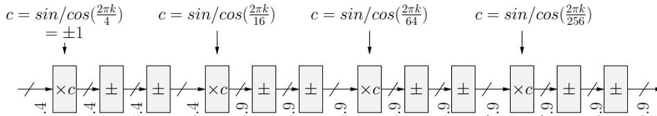
Fig. 3: Fixed-point precisions in the FFT. All the operations shown are complex operations.
