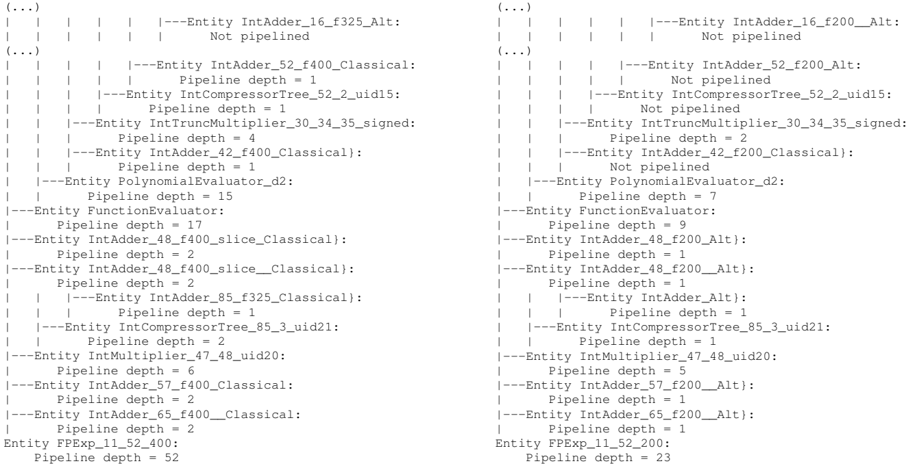
Fig. 7. Component hierarchy for e^x DP, on a Virtex4 for frequency left) f = 400MHz , right) f = 200MHz
