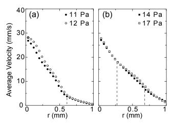
Fig. 6. Time-averaged velocity profiles for different shear stresses in the shear-thickening regime measured in the stress-controlled mode. r denotes the radial distance to the rotor; r = 0 at the rotor and r = 1 at the stator. Dotted vertical lines indicate position of the interface between the radial bands.
