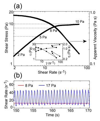
Fig. 3. Color online: (a) Flow curve of 40 mM CPyCl-NaSal solution  $(1 < \tau < 10 \text{ Pa})$  with 1 wt% tracer particles recorded under controlled shear stress conditions. The inset shows the full flow curve including the shear thickening region. Horizontal dotted lines represent the stresses where the steady state UVP velocity profiles were recorded. (b) Transient shear rate signals below (8 Pa) and above (17 Pa) shear-thickening regime of flow.
