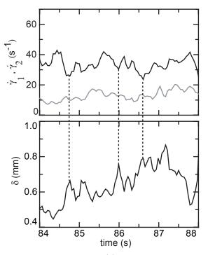
Fig. 8. Local shear rates  $(\dot{\gamma}_1, \dot{\gamma}_2)$  and position of the interface  $(\delta)$  as a function of time for a shear stress of 14 Pa. The black and the gray lines on the top part of the figure correspond respectively to the highly sheared band  $(\dot{\gamma}_1)$  near the rotor and to the weakly sheared band  $(\dot{\gamma}_2)$  near the stator.
