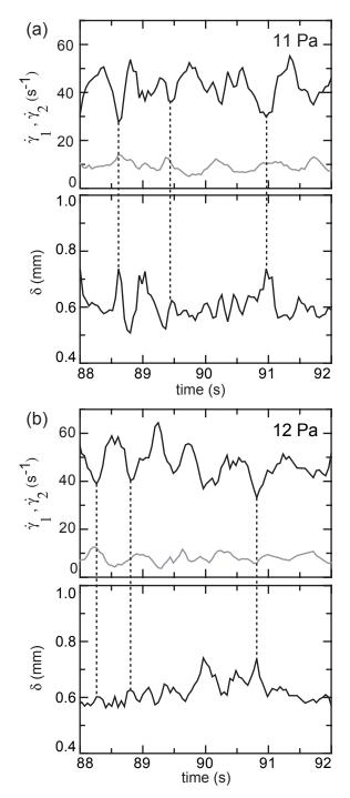
Fig. 7. Local shear rates  $(\dot{\gamma}_1, \dot{\gamma}_2)$  and position of the interface  $(\delta)$  as a function of time for (a) 11 Pa and (b) 12 Pa. The black and the gray lines on the top section of each figure correspond respectively to the highly sheared band  $(\dot{\gamma}_1)$  near the rotor and to the weakly sheared band  $(\dot{\gamma}_2)$  near the stator.
