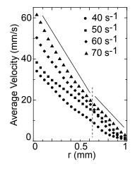
Fig. 11. Time-averaged velocity profiles for different shear rates in the shear-thickening regime measured in the strain-controlled mode. The dotted vertical line indicates the position of the interface between the radial bands and the solid lines are guides to the eye. r denotes the radial distance to the rotor; r = 0 at the rotor and r = 1 at the stator.
