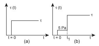
Fig. 4. Rheological test sequence used to measure velocity profiles. (a) Step stress method for shear stresses  $\tau \leq 10$  Pa and (b) Pre-shear and step stress method for shear stresses  $\tau > 10$  Pa;  $t_1 = 40$  s.
