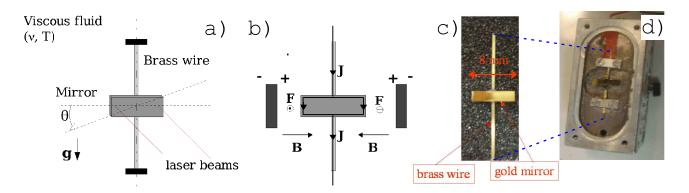
Figure 3: a) The torsion pendulum. b) The magnetostatic forcing. c) Picture of the pendulum. d) Cell where the pendulum is installed.
