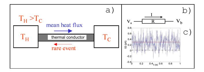
Figure 1: a) Schematic representation of a conductor whose extremities are in contact with two heat baths at temperature  $T_H$  and  $T_C$  with  $T_H > T_C$ . b) Electrical analogy. A conductor of electrical resistance R and kept at a temperature T is submitted to a potential difference  $V = V_a - V_b$ . c) Instantaneous current I flowing into the resistance using  $R = 10 \text{ M}\Omega$ , T = 300 K and  $\tau_0 = 2 \text{ ms}$ .
