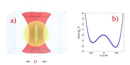
Figure 12: a) Drawing of the polystyrene particle trapped by two laser beams whose axis distance is about the radius of the bead. b) Potential felt by the bead trapped by the two laser beams. The barrier height between the two wells is about  $2k_BT$ .
