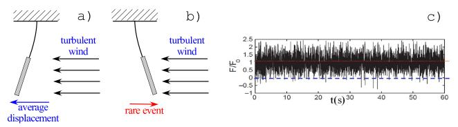
Figure 2: a)and b) Schematic representation of an object suspended by an elastic beam and submitted to the pressure of a turbulent wind a) average behavior b) rare event. c) Time evolution of the measured instantaneous force exerted by the turbulent wind on the object. The details of this experiment can be found [4]
