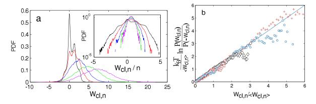
Figure 14: a) Distribution of classical work  $W_{cl}$  for different numbers of period n=1, 2, 4, 8 and 12 (f=0.25 Hz). Inset: Same data in lin-log. b) Normalized symmetry function as function of the normalized work for n=1 (+), 2 ( $\circ$ ), 4 ( $\diamond$ ), 8 ( $\triangle$ ), 12 ( $\square$ ).
