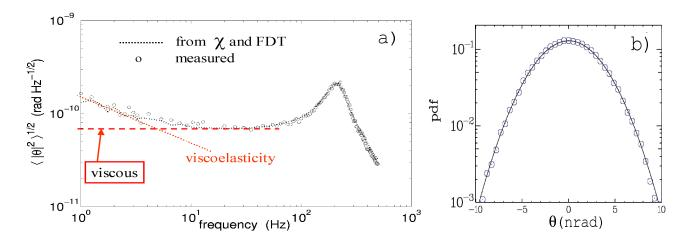
Figure 4: Equilibrium: The pendulum inside a glycerol-water mixture with M=0. a) Square root of the power spectral density of  $\theta$ .  $\circ$  directly measured spectrum, black dotted line is the spectrum estimated from the measure of  $\chi$  and using eq.3 The red dashed and dotted lines show the viscous and viscoelastic component of the damping respectively. b) Probability density function of  $\theta$ . The continuous line is a Gaussian fit
