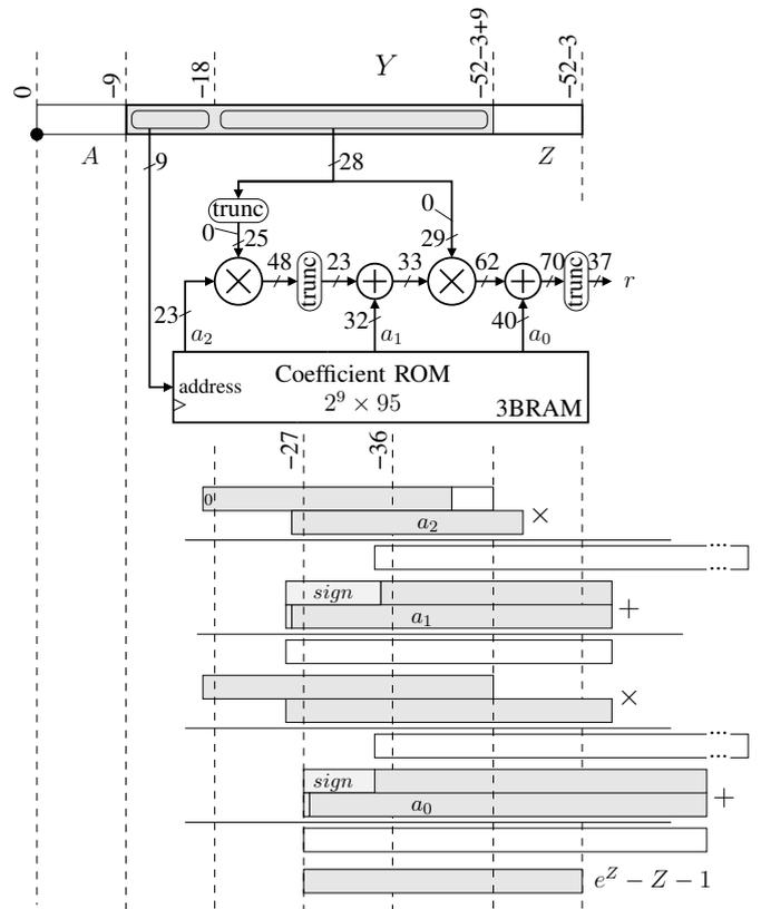
Fig. 2. The architecture evaluating  $e^Z - Z - 1$  for Virtex-5/Virtex-6
