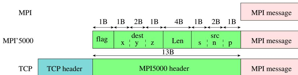
Figure 6: MPI5000 header
