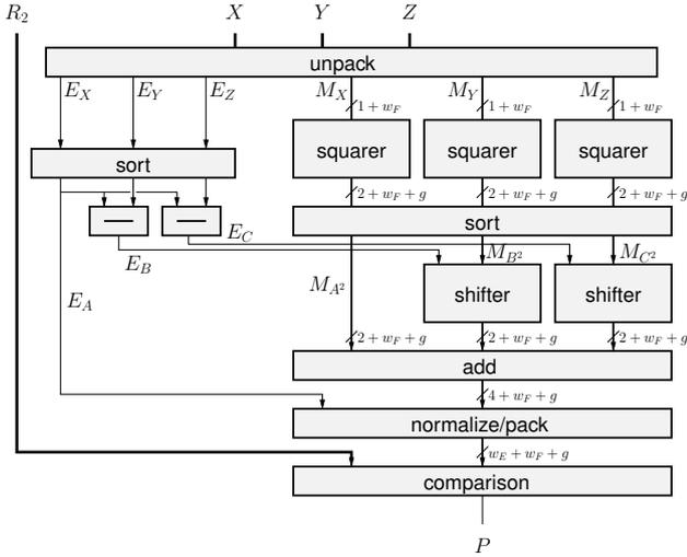
**Fig. 1.** Overview of the custom floating-point collision operator.
