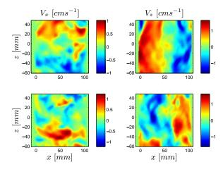
FIG. 9: Two typical instantaneous maps of the two velocity components algebraic values. Note that the color code is not the same for  $v_x$  and  $v_z$ . Top:  $\epsilon = +1$ ; Bottom:  $\epsilon = -1$  (see text).
