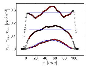
FIG. 13: The Reynolds stresses  $\tau_{xx}$  ( $\circ$ ),  $\tau_{zz}$  ( $\bigtriangledown$ ), and  $\tau_{xz}$  ( $\triangle$ ), versus x, for the lowest power (93W). The full symbols correspond to the range of the fit ( $x_{-} = 7$ mm,  $x_{+} = 94$ mm). The lines show the proposed fit.
