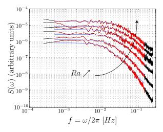
FIG. 5: The spectra of the bridge output, for various Ra values (second cell, Pr = 6). The lines correspond to the fit used for extracting  $\tau_o$ . The range for the fit is signaled in red on the spectrum.
