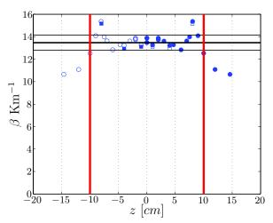
FIG. 6: Temperature gradient versus the height in the cell, for the second cell. Only full symbols correspond to real measurements. Open symbols are simply symetric to the full ones compared to the middle of the cell. The two vertical bars signal the ends of the channel. The thick horizontal line stands for the average of  $\beta(z)$  in the center of the channel. The lower and upper horizontal lines correspond to  $\pm 5\%$  of this mean value.
