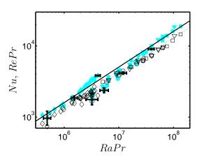
FIG. 7: Evolution of Nu (full symbols) and RePr (open symbols) versus RaPr. First cell:  $\circ$ , Pr = 6.6;  $\bigtriangledown$ , Pr = 5.3;  $\Box$ , Pr = 4.1. Second cell:  $\diamond$ , Pr = 6. Full line, proposed average law for Nu results:  $Nu = 1.6\sqrt{RaPr}$ . Dotted line, proposed average law for RePr results:  $RePr = 1.3\sqrt{RaPr}$
