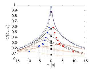
FIG. 3: The correlation function  $C(\delta z, \tau)$  for various  $\delta z$  in the high power case (235W). The dots correspond to the position of the highest peak and its symetric compared to  $\tau = 0$ . The squares mark the value of  $C(\delta z, 0)$  for the different  $\delta z$ , from the darker to the lighter: 4mm, 10mm, 20mm, 30mm, 40mm, 50mm (twice), 60mm, 70mm, and 100mm. The blue (top) curve corresponds to the autocorrelation of one sensor (*i.e.*  $\delta z = 0$ ).
