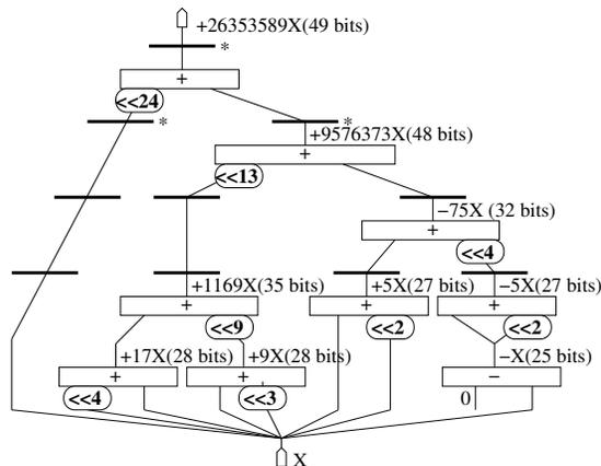
Figure 1: Multiplier by 26353589 pipelined for 200MHz.
