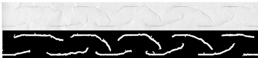
FIG. 2 – Post-mortem images of a fractured sample with  $d = 1.5\text{cm}$  : at the top, initial digitized image and, at the bottom, corresponding binary image with extracted crack paths obtained through image processing.
