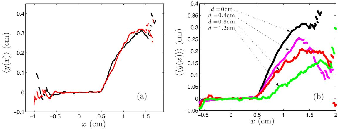
FIG. 11 – Paths of repelled cracks (type B). (a) Average crack profile  $\langle y(x) \rangle$  for two samples with  $d = 1\text{cm}$ , and (b) average crack profile  $\langle\langle y(x) \rangle\rangle$  for four value of  $d$ .
