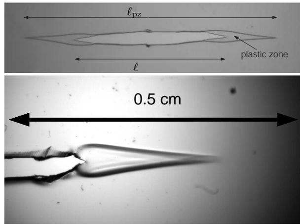
**Fig. 3.** On top : image of a crack in a polycarbonate film with its macroscopic plastic zone at each tip.  $\ell$  is the crack length and  $\ell_{pz}$  is the plastic zone length from tip to tip. At the bottom : plastic zone at the tip of a growing crack in a polycarbonate film.
