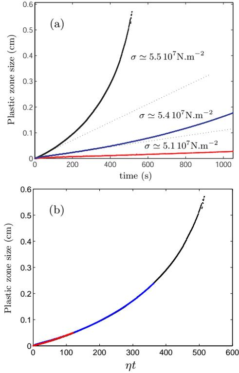
**Fig. 7.** Plastic zone size as a function of (a) time and (b) rescaled time for three experiments performed with different applied stresses. Constant  $\eta$  is defined with an arbitrary prefactor in order to make the growth curves collapse.
