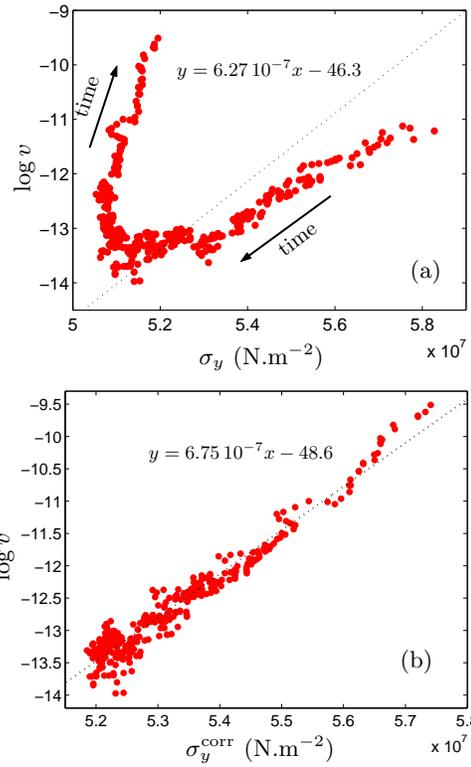
**Fig. 15.** Natural logarithm of the instantaneous crack growth velocity as a function of (a) the Dugdale-Barenblatt stress and (b) the corrected Dugdale-Barenblatt stress  $\sigma_y^{\text{corr}}$  for an experiment performed with  $F = 900\text{N}$  and  $\ell_i = 1.5\text{cm}$ . In Fig. (a), the dotted line is the result of the Fig. 14 data fit. In Fig. (b), the dotted line is the result of a linear data fit.
