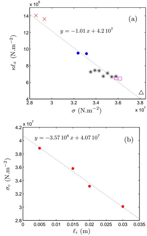
**Fig. 17.** (a)  $\kappa\ell_x$  for various experimental conditions ( $\ell_i = 1.5, 2, 3\text{cm}$  and  $2.9 < \sigma < 3.8 \cdot 10^7 \text{N.m}^{-2}$ ) as a function of the applied stress  $\sigma$ . (b) Critical rupture stress  $\sigma_c$  as a function of the initial crack length  $\ell_i$ . The dotted lines are a linear fit of the data.
