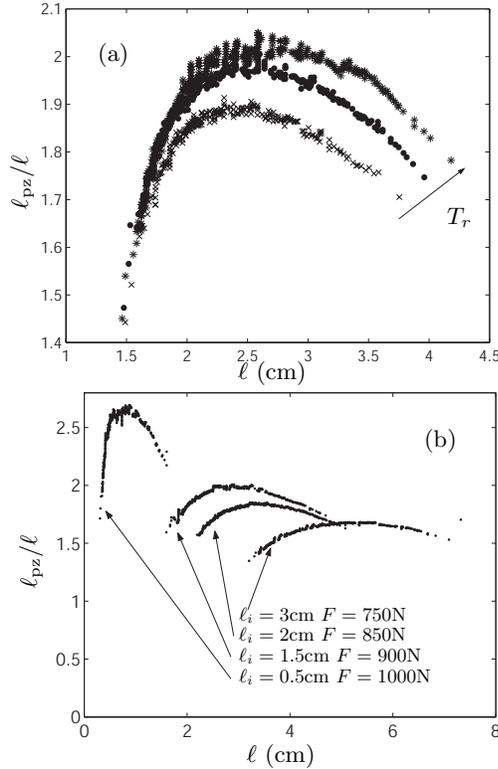
**Fig. 13.**  $l_{pz}/\ell$  ratio as a function of the crack length (a) for three experiments performed with the same experimental conditions ( $l_i = 1.5\text{cm}$  and  $F = 900\text{N}$ ), (b) for four experiments performed with different experimental conditions.
