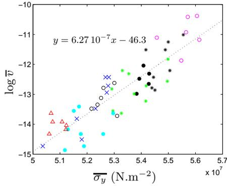
**Fig. 14.** Natural logarithm of the average crack growth velocity  $\bar{v}$  as a function of the average plastic stress during the growth. Each point represents the average dynamical behavior during an experiment. Experimental conditions are various ( $\ell_i = 1.5, 2, 3\text{cm}$  and  $2.9 < \sigma < 3.8 \cdot 10^7 \text{N.m}^{-2}$ ). Each experimental condition corresponds to different symbols.
