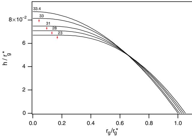
**Fig. 5.** Four normalized profiles calculated at four different temperatures for the liquid crystal 8CB. The temperature is given beside each profile. An arrow marks the edge of the facet on each profile. At 33.4 °C, the droplet has the shape of a spherical cap.
