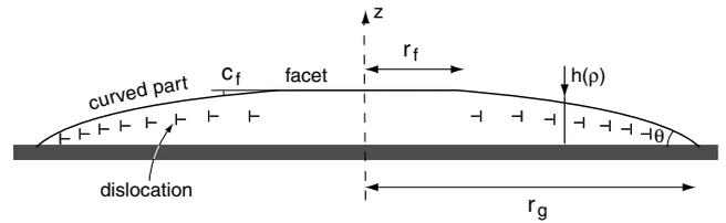
Fig. 2. Droplet configuration.
