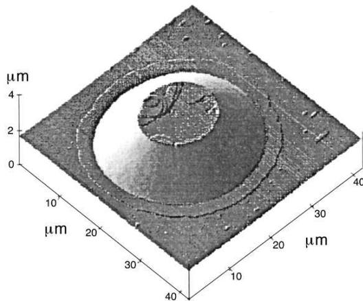
**Fig. 14.** Three-dimensional view of a droplet of the chiral liquid crystal XI/12 obtained by tapping mode atomic force microscopy. The droplet has been deposited in the smectic A phase at high temperature (about 100 °C) and then slowly cooled down to the room temperature in the SmC\* phase (from Ref. [33]).
