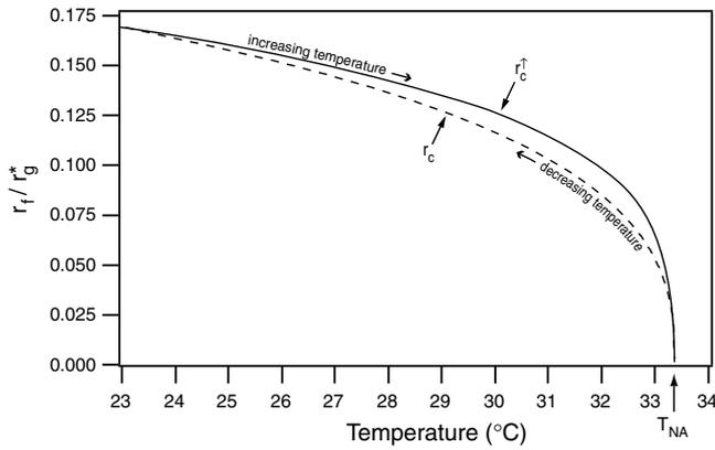
**Fig. 8.** Radius of the facet as a function of the temperature at increasing temperature (solid line, curve  $r_c^{\uparrow}$ ). For comparison, we reported the critical radius as a function of the temperature (dashed line, curve  $r_c$ ).
