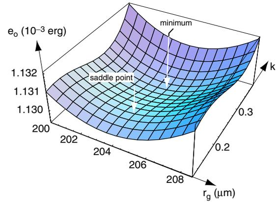
**Fig. 4.** 3D plot of the droplet energy  $e_o$  as a function of  $k = r_f/r_g$  and  $r_g$ . The saddle point and the absolute minimum are indicated by two arrows (8CB,  $T = 24^\circ\text{C}$ ,  $V = 10^{-6} \text{ cm}^3$ ).
