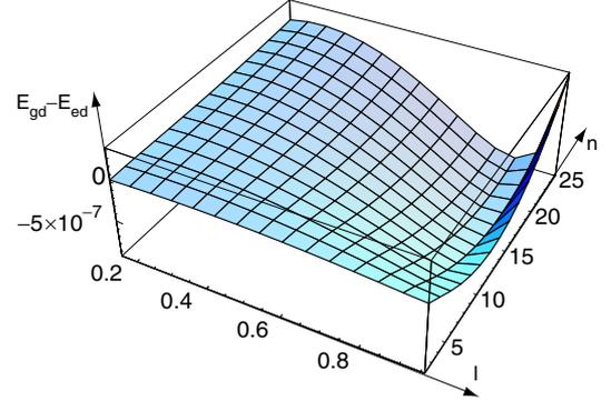
**Fig. 12.** Plot of the difference energy  $E_{gd} - E_{ed}$  as a function of  $n$  and  $l = \delta/r_g$  calculated for 8CB at  $T = 24^\circ\text{C}$ . In this graph,  $l_{min} \approx 0.39$  and  $n_{min} \approx 14$ , while  $l_{opt} \approx 0.87$  and  $n_{opt} \approx 16$ .
