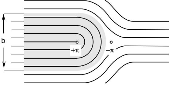
**Fig. 11.** Giant dislocation. The core is decomposed into a pair of  $(\pm\pi)$ -wedge disclination lines. These two lines have a singular core. This model was first proposed by Williams and Kléman [32].
