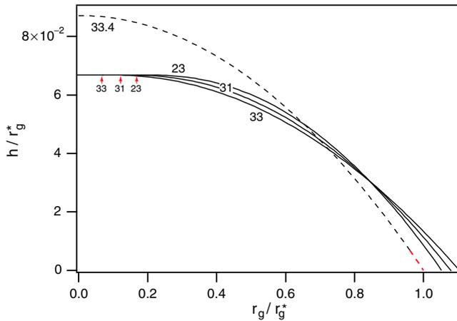
**Fig. 9.** Evolution of the droplet profile when the temperature is increased. The temperature is indicated beside each profile and an arrow marks the edge of the facet. Although the droplet height does not change, the facet radius decreases. Because the volume is conserved, the droplet radius increases. The dashed line corresponds to the droplet profile in the nematic phase (spherical cap).
