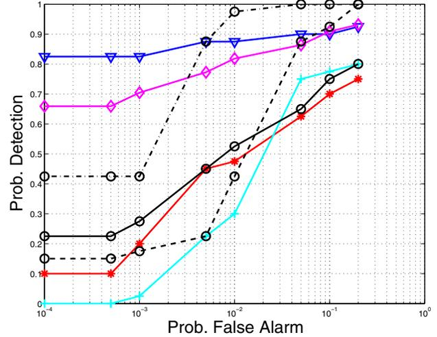
**Figure 3. DETECTION VS. FALSE ALARM RATES.  $T = 1$ min. For distance  $D_\alpha$  and for attacks #3(7%,\*), 4(12%, $\nabla$ ), 6(10%,+), 7(27%, $\diamond$ ), 8(4%,o) in Table 1. For 8(4%,o), dashed and mixed lines correspond to  $K_{\Delta}^{1d}$ , with  $\Delta = 10$ ms and  $\Delta = 40$ ms, for comparison.**
