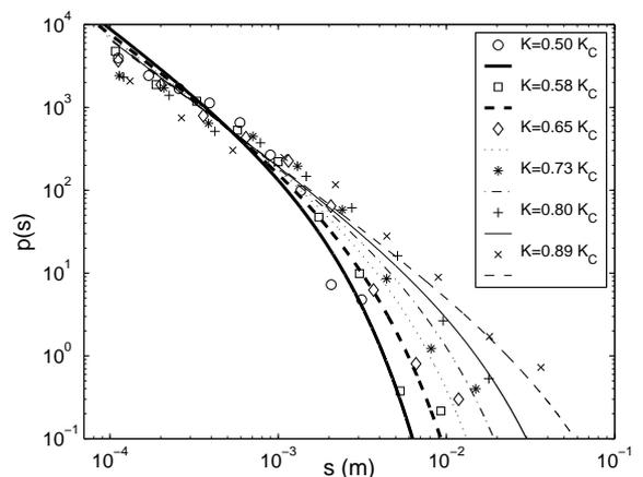
FIG. 2: Probability distribution of step sizes for various values of stress intensity factor. Choosing  $\lambda = 50\mu\text{m}$ , the different curves are the best fits of eq.3 giving an average value  $V = 5 \pm 1 \text{ \AA}^3$ .
