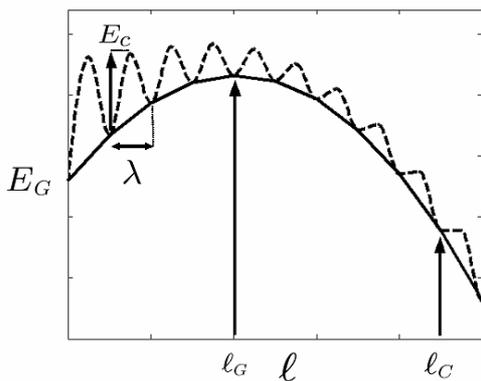
FIG. 3: Sketch of the Griffith potential energy  $E_G$  as a function of crack length  $\ell$  with constant applied stress (solid line). The energy barriers  $E_C$  and the discretization scale  $\lambda$  are represented by the dashed curve.
