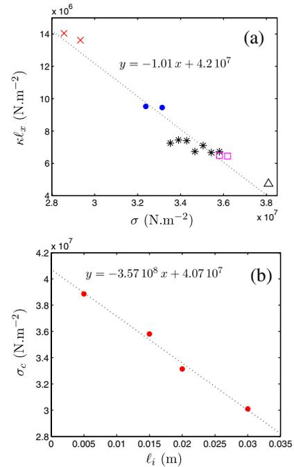
FIG. 6 (color online). (a)  $\kappa \ell_x$  for various experimental conditions ( $\ell_i = 1.5, 2, 3$  cm and  $2.9 < \sigma < 3.8 \times 10^7$  N m $^{-2}$ ) as a function of the applied stress  $\sigma$ . (b) Critical rupture stress  $\sigma_c$  as a function of the initial crack length  $\ell_i$ . The dotted lines are a linear fit of the data.
