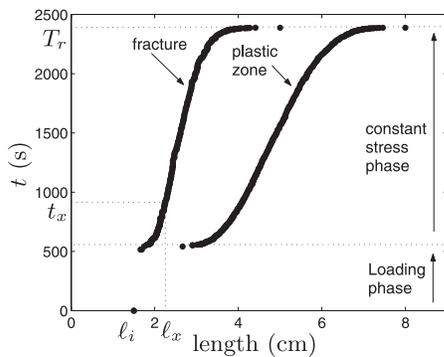
FIG. 2. Time as a function of both the crack and process zone lengths for an imposed stress experiment ( $\ell_i = 1.5 \text{ cm}$ ,  $F = 900 \text{ N}$ ). We indicate the position of the inflection point ( $t_x$ ,  $\ell_x$ ) of the crack growth curve.
