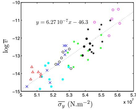
FIG. 4 (color online). Natural logarithm of the average crack growth velocity  $\bar{v}$  as a function of the average plastic stress during the growth. Each point represents the average dynamical behavior during an experiment. Experimental conditions are various ( $\ell_i = 1.5, 2, 3$  cm and  $2.9 < \sigma < 3.8 \times 10^7$  N m $^{-2}$ ). Each experimental condition corresponds to different symbols.
