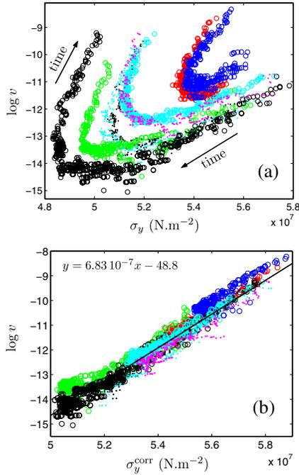
FIG. 5 (color online). Natural logarithm of the instantaneous crack growth velocity as a function of (a) the Dugdale-Barenblatt stress, (b) the corrected Dugdale-Barenblatt stress  $\sigma_y^{\text{corr}}$  according to Eq. (3) for eight experiments performed with various experimental conditions ( $\ell_i = 1.5, 2, 3$  cm and  $2.9 < \sigma < 3.8 \times 10^7$  N m $^{-2}$ ). In Fig. (b), the black line is the result of a linear data fit.
