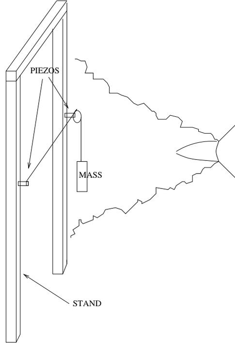
**Figure 1.** Eperimental setup: the thin steel wire is pulled across a turbulent air jet by a 4 Kg weight on a rigid stand. Piezoelectric transducers are in mecanical contact with the wire at each end.
