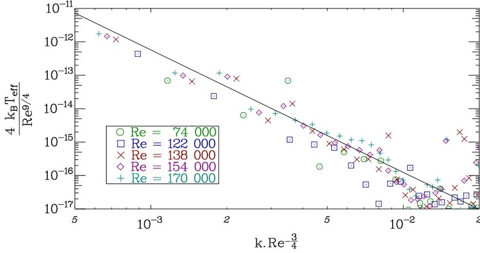
**Figure 4.** Spectrum of the FDR, labelled as *thermal agitation* per degree of freedom. Axis are rescaled with proper Reynolds number dependence, between 74000 and 170000. The size of the symbols represents the uncertainty in the determination of the maxima of the peaks. The solid line is a  $k^{-11/3}$  power-law given as an eye guide.
