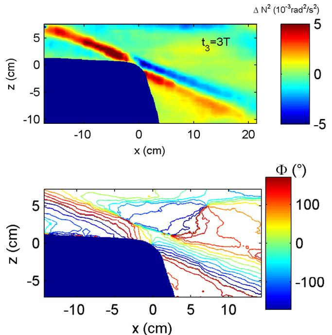
FIG. 2: (Color online) Panel a presents the two-dimensional vertical density gradient, while panel b shows the phase. Both plots have been averaged over one tidal period of the experiment around  $t = 3T$ . Horizontal and vertical distances are in cm. The generation point C appears to be an amphidromic point around which the phase of the wave rotates.
